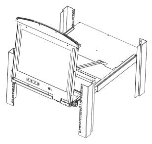
4. Reach underneath and pull the keyboard module all the way out until it clicks into place.
